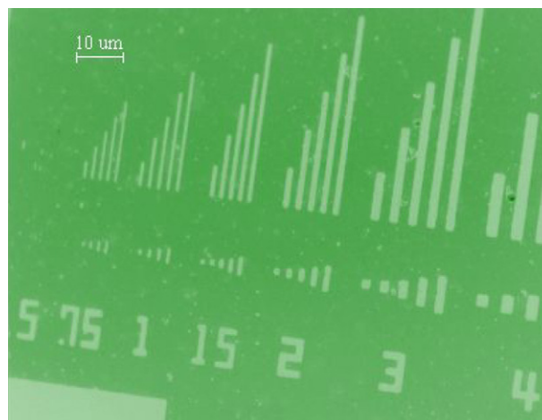
Fig. 14. Optical micrograph of positive fine patterns with p(DDMA/NPMA/TsPMA)s c LB film 35 layers on a glass substrate after UV irradiation following development with 1% TMAH aqueous solution.
